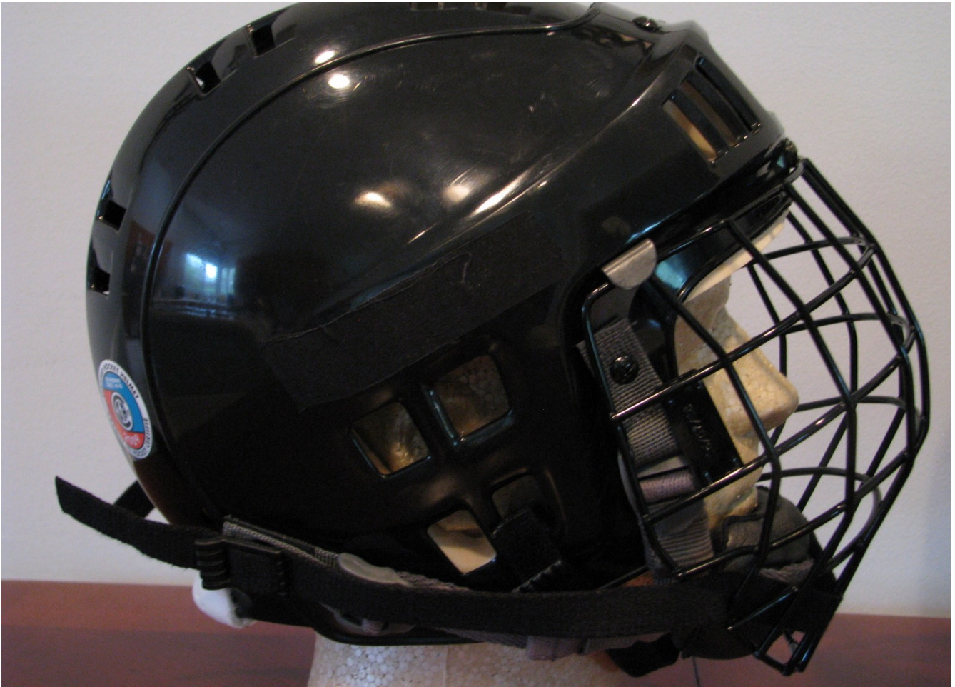
Figure 10 Helmet A with 4 point chin strap installed and cage straps fastened. It does not change the appearance of the helmet. This chin strap system using a slide buckle load tests to 215 ft lbs on military helmets* before buckle failure and will improve helmet retention. However it may not prevent all helmet loss.
