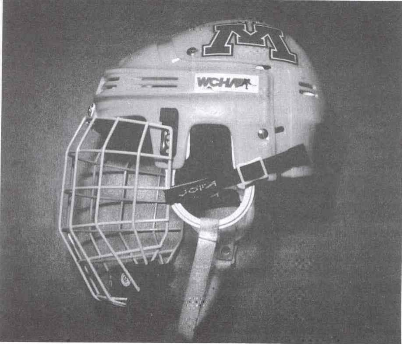
Figure 3 (Single chin strap mandated by the HECC's selection of the ASTM helmet standard)
