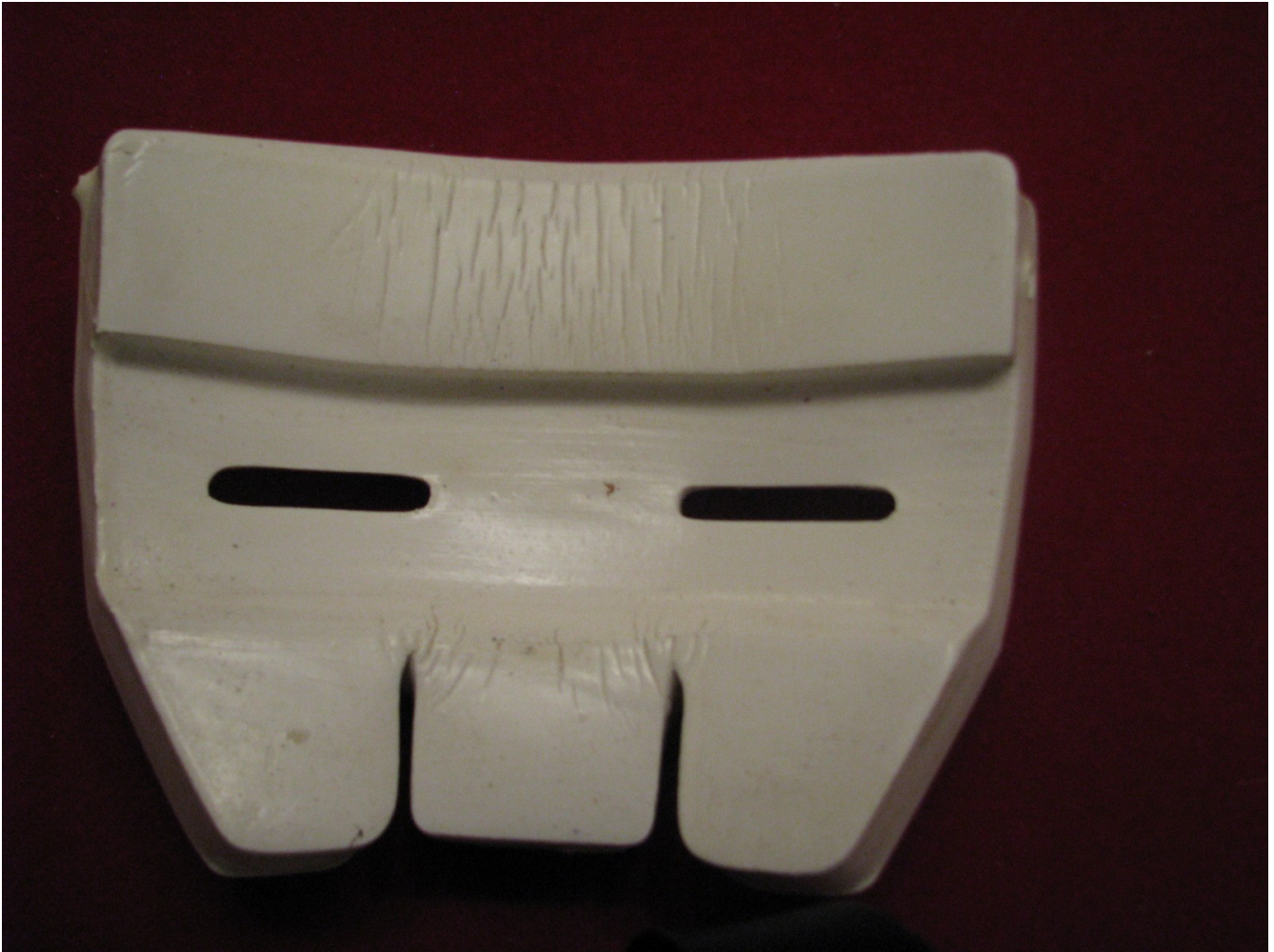
Fig 16 Flat pad removed from football helmet. Compression set of pad clearly visible.
