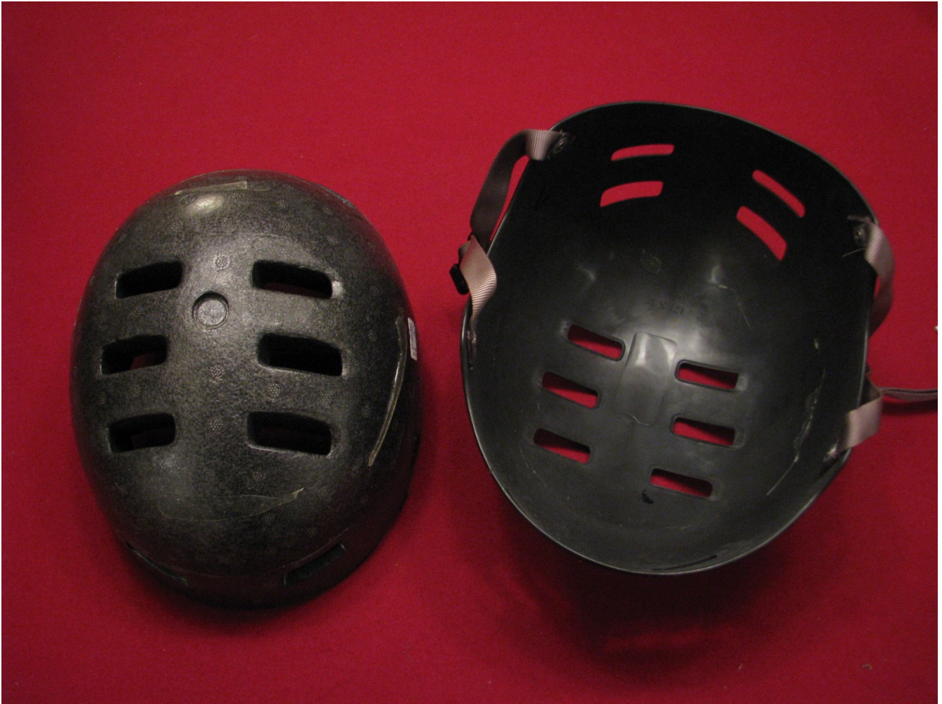
Figure 15 Multi sport helmet with a molded liner (removed) < 1mm liner to shell gap.
