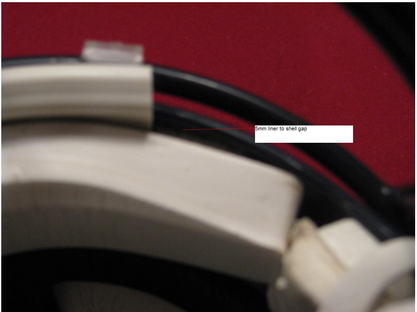
Figure 12 Football helmet flat liner to shell 5mm gap.
