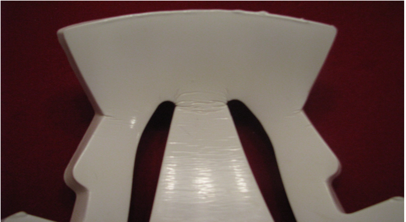
Fig 14 Flat pad removed from lacrosse helmet. Compression set of flat pad clearly visible.
