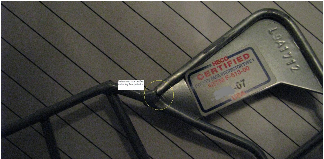
Fig 20 Failed HECC certified cage
