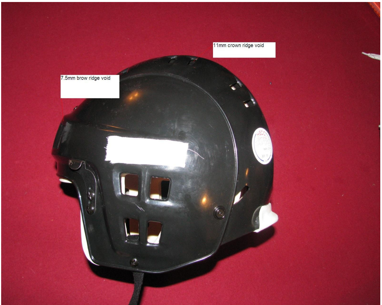
Figure 11 Voids in ice hockey helmet.
