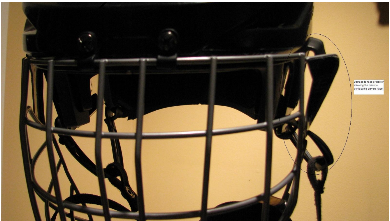
Fig 21 Failed HECC certified cage failure front view.
