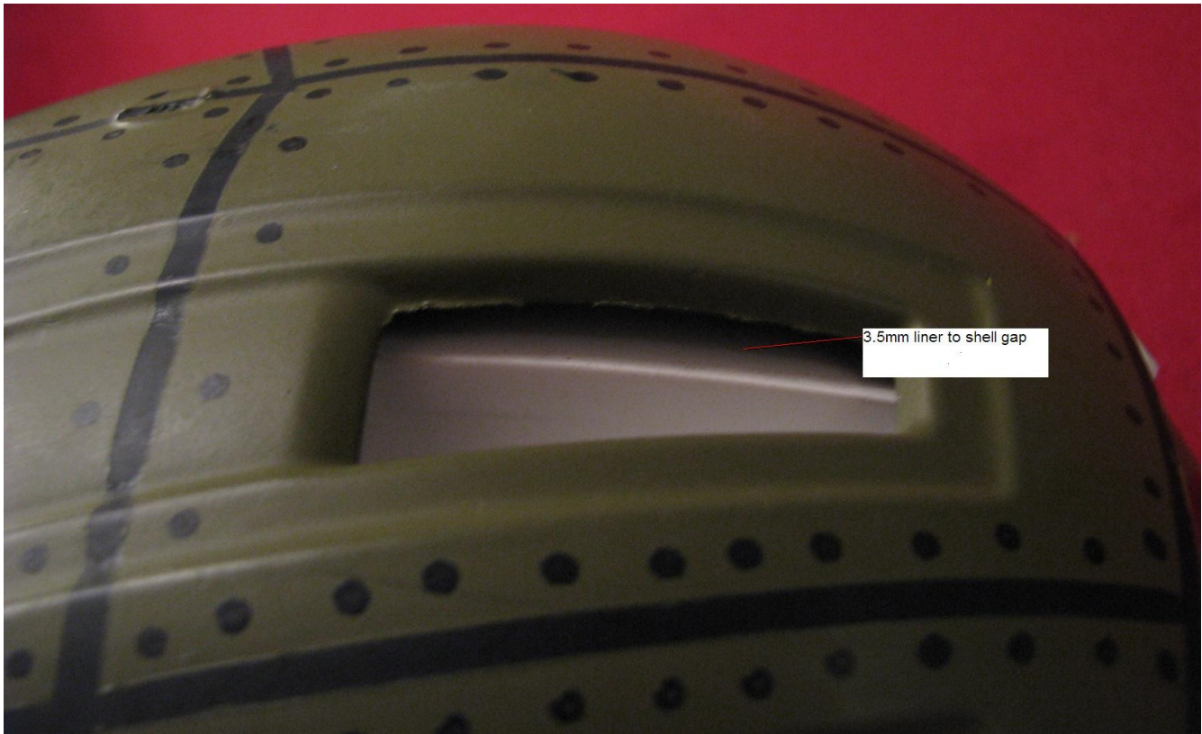
Figure 9 Lacrosse helmet flat liner pad to helmet shell 3.5mm gap.
